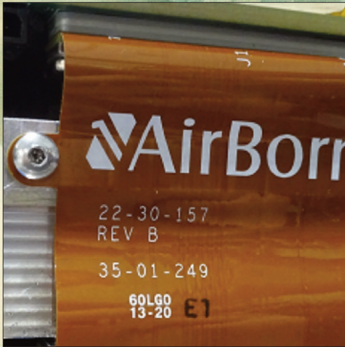
Figure 2 – Fully assembled configuration. A stainless steel stiffening plate applied between the fasteners secures the flex cable and the flexible PCB to provide uniform compression along the interconnect.
